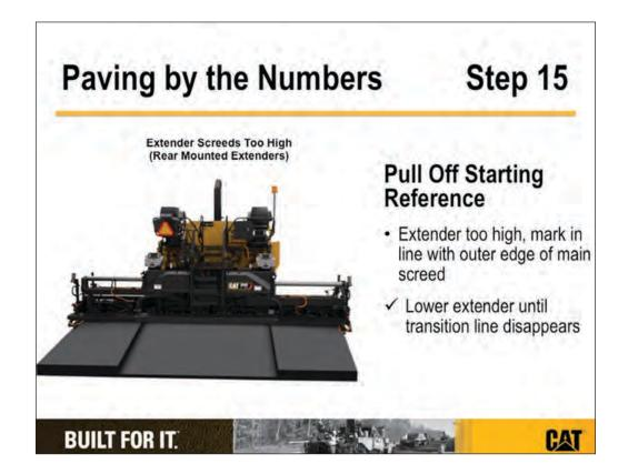
If an extender is set too high, there will be a longitudinal transition mark in line with the outer edge of the main screed. The mat will be thicker behind the screed extender.
