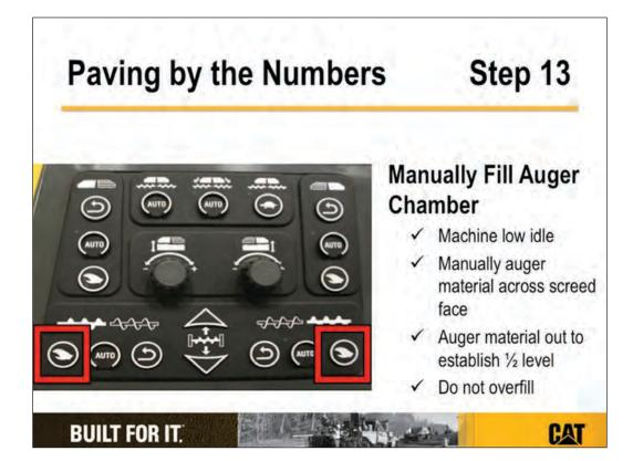
Then, use the manual auger switch to move material out to the end of the screed. The correct head of material covers one half of the augers.
