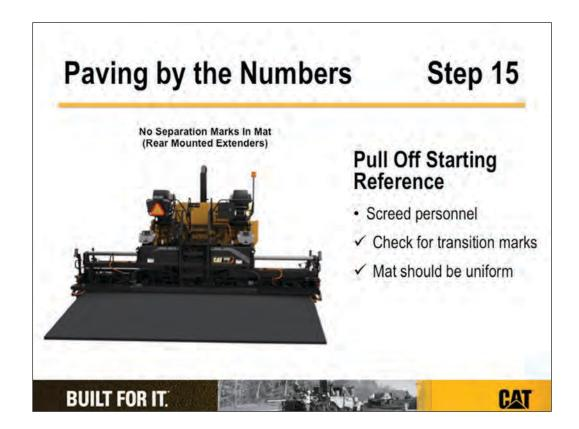
As paving speed and feeder system operation are stabilized, screed personnel should look for transition marks between the main screed and screed extenders.
