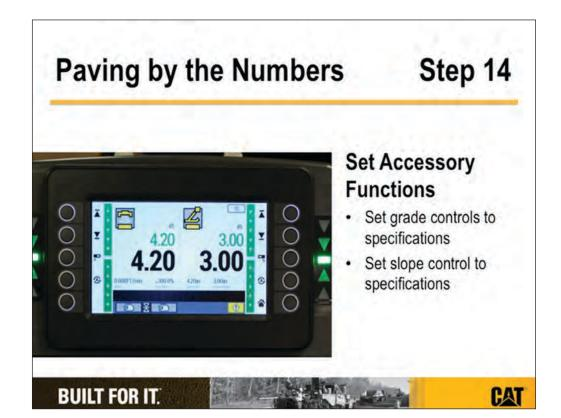
Automatic grade and slope controls are considered accessory controls. Set them according to to the job specifications. Install any averaging devices and controls as required.
