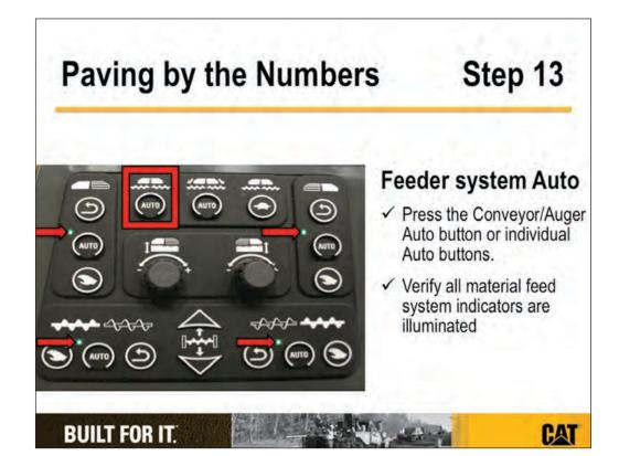
When you have filled the auger chamber half full—no more, no less—put the conveyor and auger mode switches on the operator's console to Auto. Either push the automatic conveyor and auger button or press individual automatic buttons for both the conveyor and auger. Verify that all four automatic system indicators are illuminated.
